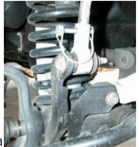
Trim the factory axle bracket off approx 40%. Weld new sway bar extension bracket next to old bracket. Fig.14
