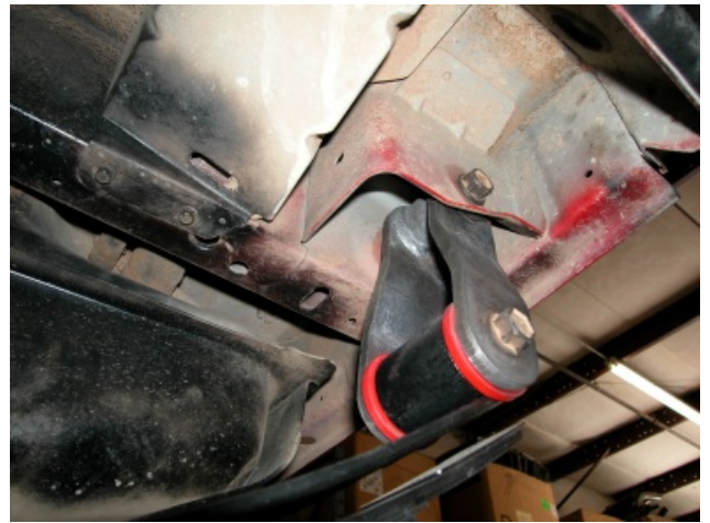
Rear Shackle and leaf spring installed.
