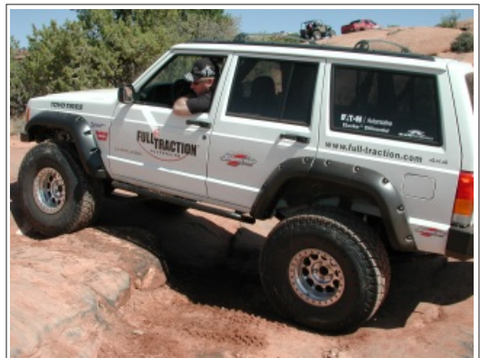
Full-Traction 6" Long Arm on 35" x12.50 Tires
